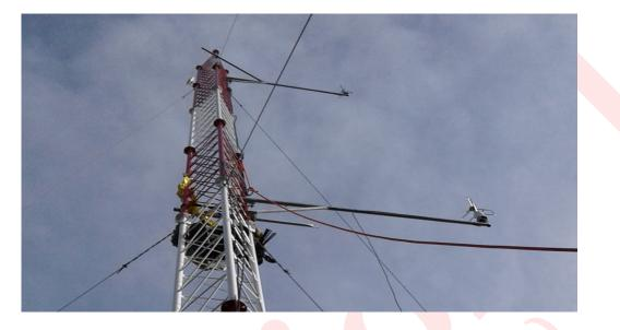
Figure 2: Tower (N. 41/riNE02) with sonics (RMY81000) mounted vertically at the end of the booms.
